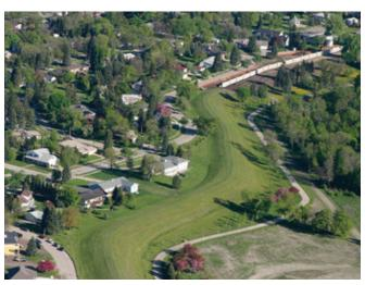
A permanent levee and floodwall system protecting Grand Forks, ND. Image: FEMA / Brenda Riskey
