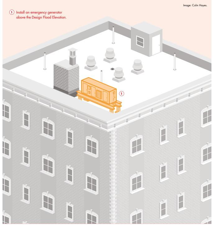
During a power outage, backup power is vital to continue building operations and make repairs during and after a storm event.
